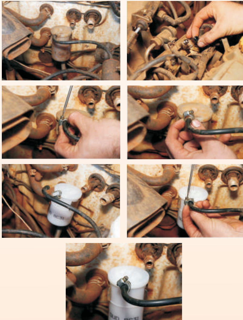
Fig: Photographs of Replacing Fuel Filter
